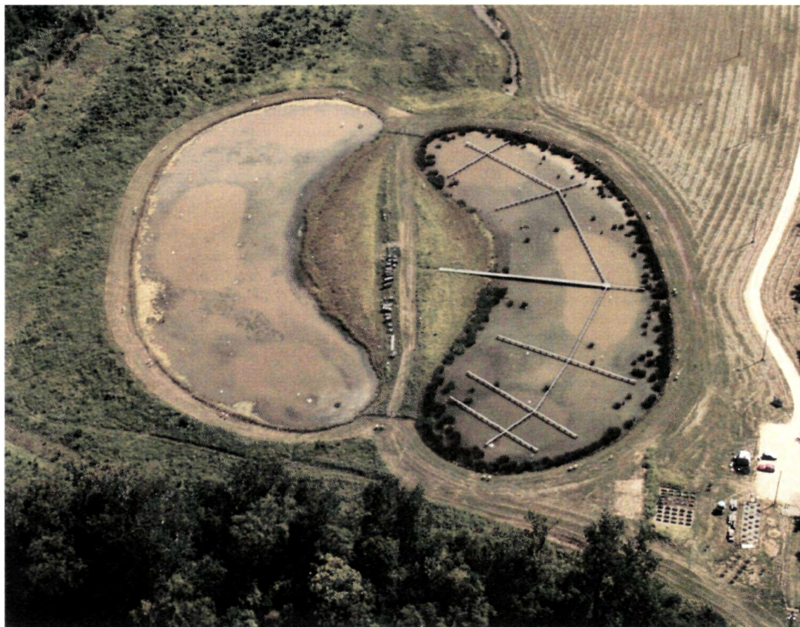
Experimenting with “nature’s kidneys” on the Ohio State University campus allows researchers to probe the complex working of wetlands. The multiyear project at the 2.5-acre Olentangy River Wetland Research Park in Columbus includes a pair of constructed wetlands, one planted in 1994 (right) and the other an unplanted control. (Photo courtesy William Mitsch, Ohio State University)
